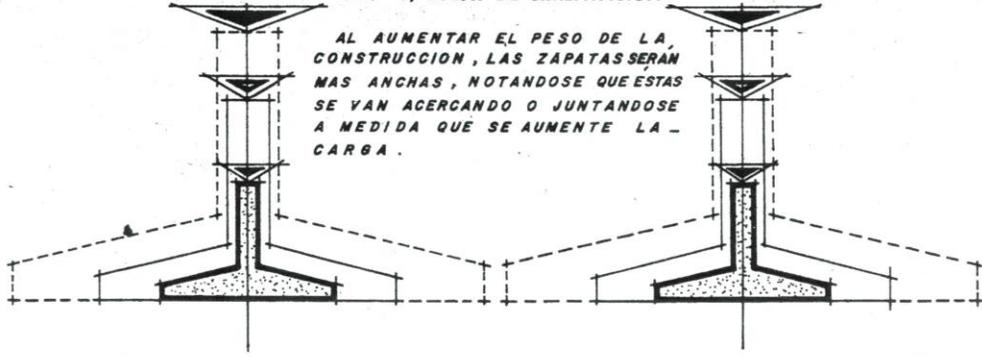
AL LLEGAR A APROXIMARSE DICHOS ELEMENTOS ESTRUCTURALES OPTAREMOS POR UTILIZAR LA LOSA DE CIMENTACION, EXISTIENDO DESDE LUEGO LAS CONTRATRABES, PARA RECIBIR LAS CARGAS CONCENTRADAS (COLUMNAS, MUROS ETC)
